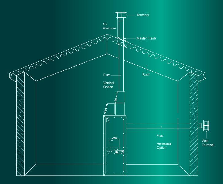
The horizontal flue installation allows for reduced flue run as there is no requirement to install the flue to the top of the building as with normal conventional flue systems, saving on time and flue materials for the installing contractor
