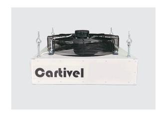
Cartivel DSF destratitification fans consist of a quiet, yet powerful, axial fan mounted on a slim box frame. Air is discharged through a 4 way adjustable louvre in the base of the frame.
